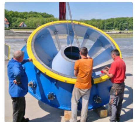
Fig. 2. Water turbine inlet with Belzona® 1341 coating
