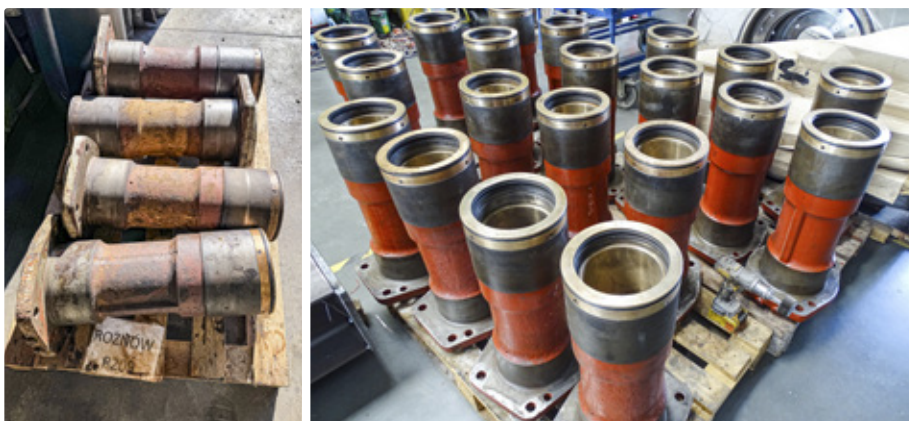
Fig. 13. Bearing sleeves before and after reconditioning
