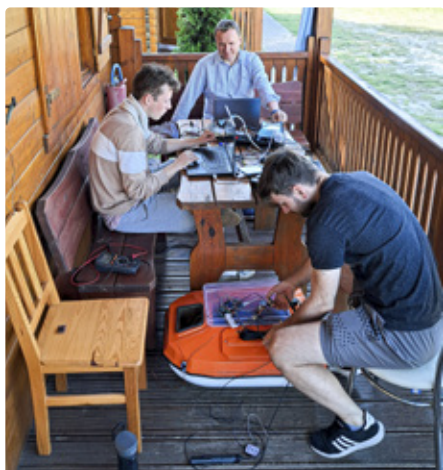
Fig. 2. Unmanned floating drone's sensors programming, tests including measurement systems calibration
