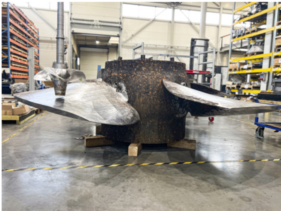
Fig. 1. The runner of the overhauled turbine, juxtaposed with an IOZE hydro runner (IOZE rivus microturbine)
