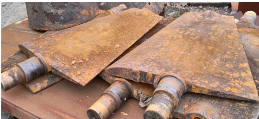
Fig. 1. Surface area of Kaplan turbine vanes after years of operation (the Oder River)
