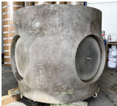
Fig. 5. Runner hub: after disassembly, after cleaning and after coating with epoxy paint
