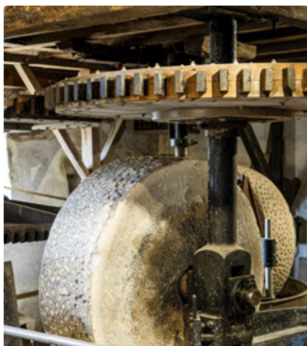
Fig. 4. The round-form machine used to grinding the raw material
