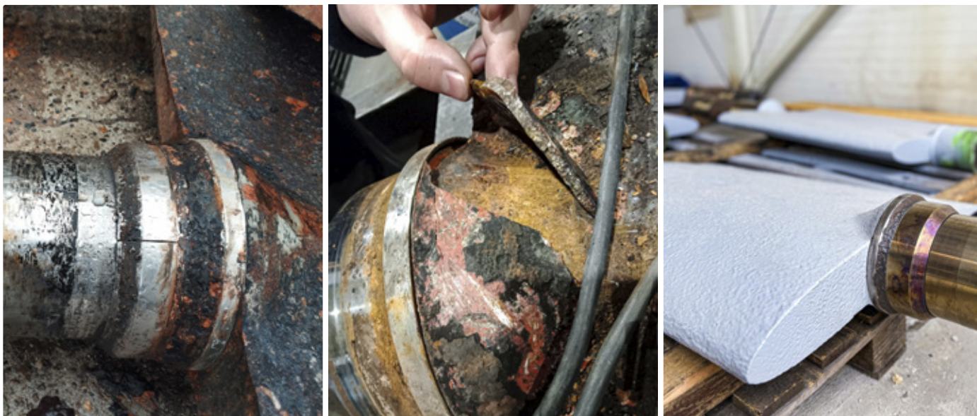
Fig. 14. The corroded stub/guide vane interface and the remanufactured workpiece
