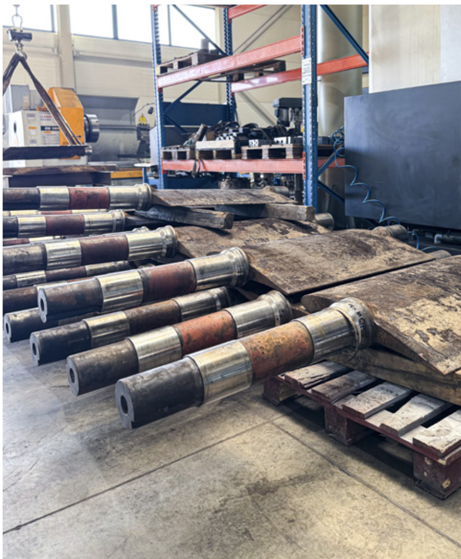
Fig. 15. Inlet guide vanes before and after overhaul
