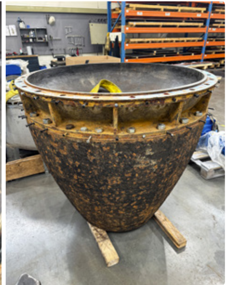
Fig. 2. Manual cleaning of the inside of the runner hub — hub cover prior to overhaul
