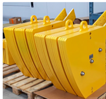
Fig. 3. The counterweight weights of DN2200 PN6 butterfly valves of individually selected shapes
