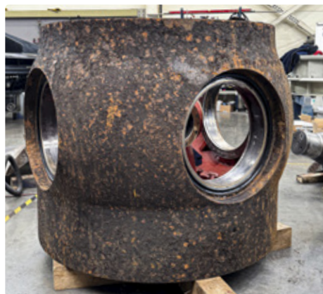
Fig. 5. Runner hub: after disassembly, after cleaning and after coating with epoxy paint
