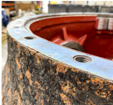
Fig. 3. Close-up of the hub surface before and after blast cleaning
