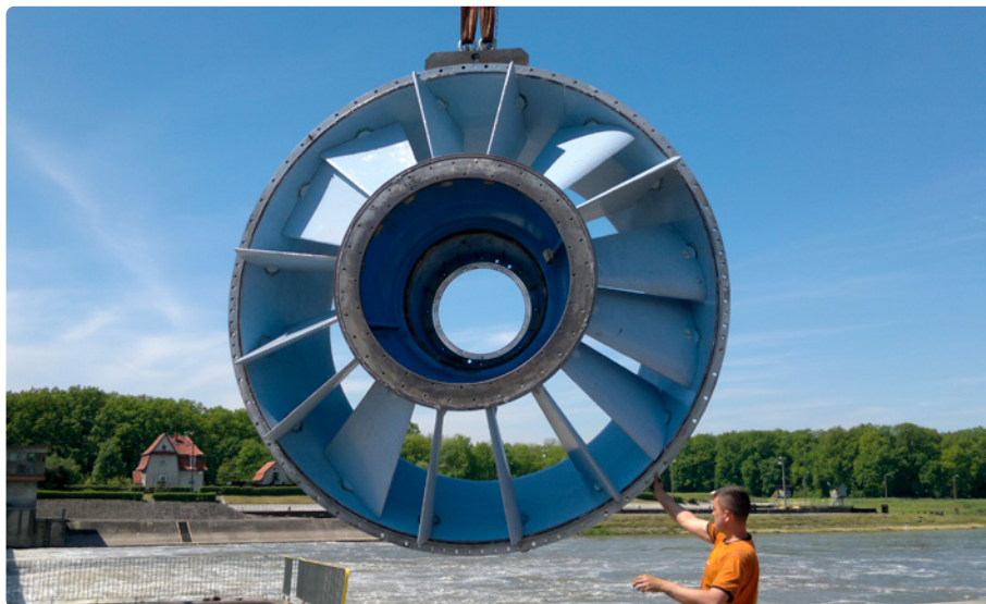
Photo 3. Kaplan turbine guide vane (on the Oder River) with BELZONA(1341) composite coating applied
