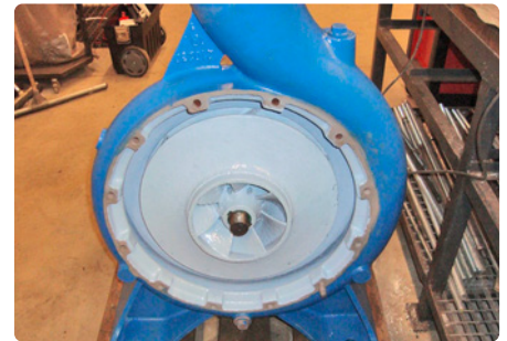
Photo 4. 90 kW pump before and after coating with BELZONA(1341)
