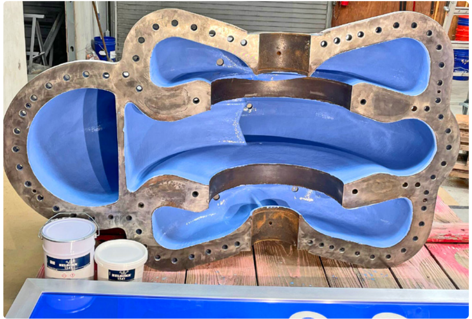
Photo 1. BELZONA(1341) SUPERMETALGLIDE, a coating whose surface is 20 times smoother than polished stainless steel
