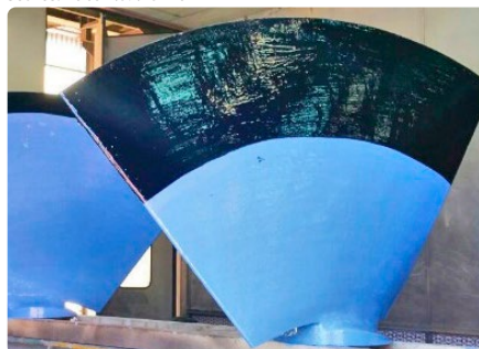
Photo 7. Water turbine runner blades covered with Belzona®1341 and Belzona®2141 hydrophobic and anti-cavitation coatings, respectively
