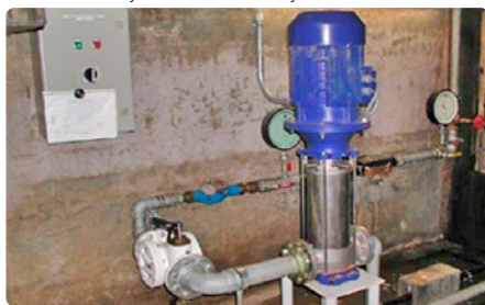
Photo 1a. Test rig used for establishing the cavitation erosion initiation period of a streamlined surface
