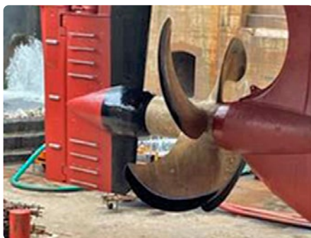
Photo 4. Belzona®2141 coating used to protect ship rudder and propeller against cavitation
