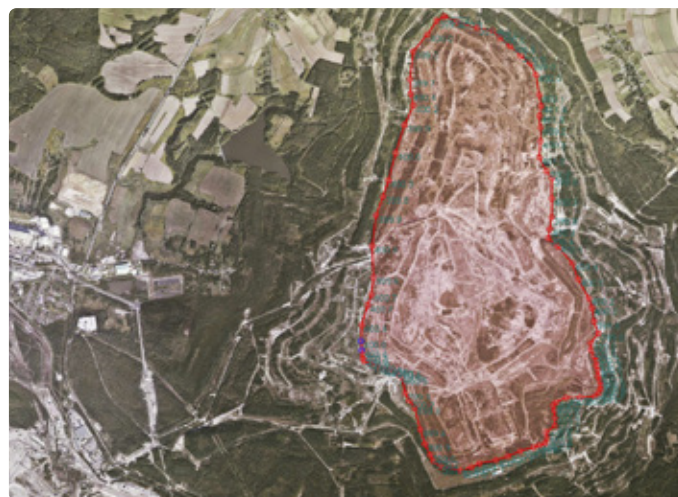
Fig. 3. Proposed location of the upper reservoir. Reservoir bottom level at 400 m above sea level, marked area is 657.58 ha.
