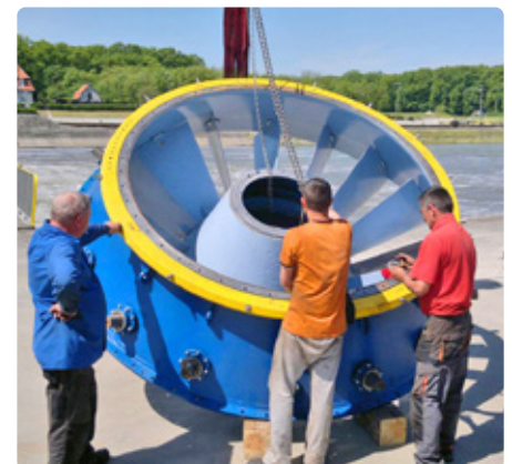
Photo 2. Water turbine inlet with Belzona® 1341 coating
