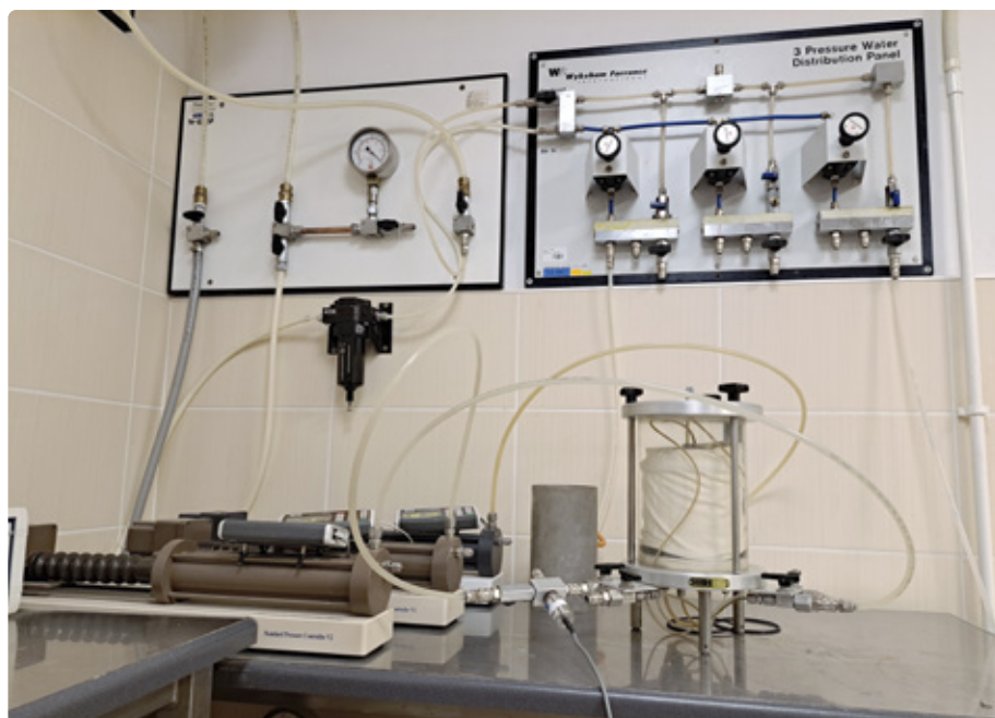
Photo 1. Set for testing the hydraulic conductivity t at specified pressure and constant head
