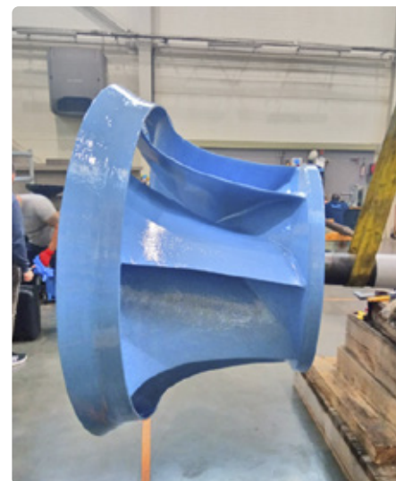
Photo 6. Water turbine rotor with Belzona® 1341 coating
