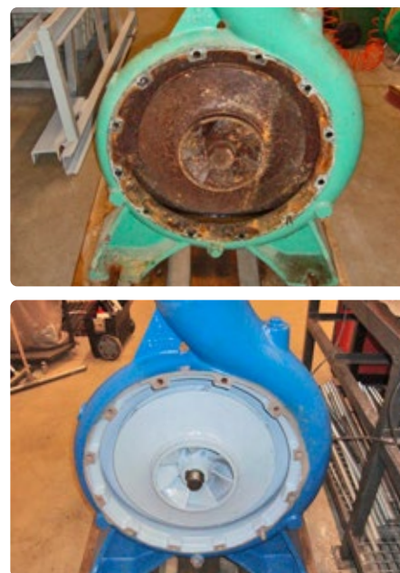
Photo 4. 90 kW pump before and after coating with BELZONA(1341)
