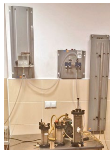
Photo. Apparatus to laboratory tests at constant head of filtration in accordance with PKN-CEN ISO/TS 17892-11 and ASTM D2434
