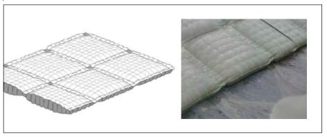
are most often found in use on river banks with susceptible and uncertain substrate. The length of the spacers ranges from 8 to 56 cm, hence the average thickness of the mat can be from 10 to 45 cm. On canals, these mats are used on the excavated sections, i.e. when there may be groundwater inflow into the canal.
