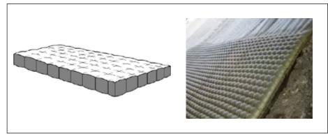
Fig. 3. Incomat® Flex (left) schematic sketch with cross section, (right) view of mattress after concrete filling, photo: Huesker.
