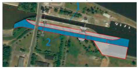
Fig. 14. Construction of additional spans with a low Jambor-type sill [8]; 1 – the existing spans of the Włocławek weir; 2 – additional spans of the weir with a Jambor-type sill; 3 – front dam.
