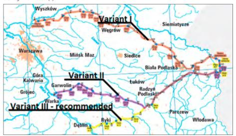
Fig. 6. Route of the planned Deblin – Brest canal within the E40 waterway in accordance with stage III of the study [3].
