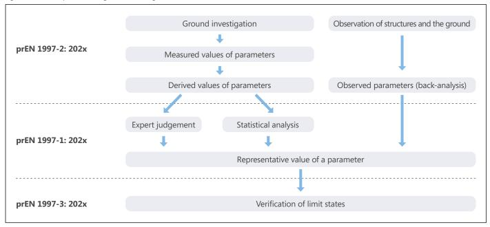
Fig. 5. Sheme for determining the representative value of a soil parameter in the geotechnical design process [9].
