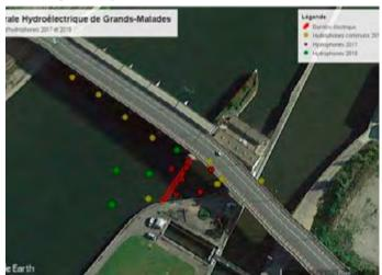
Fig. 6. 2D telemetry network at CHR. Certain receiver positions have changed from 2017 and 2019: common items are in yellow, 2017 items are in red and 2019 items are in green (Sonny et al. 2020).
