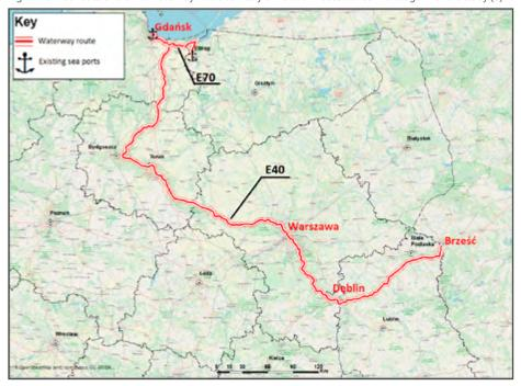
Fig. 3. The planned route of the E40 waterway on the Vistula River in accordance with variant II of stage III of the study [3].
