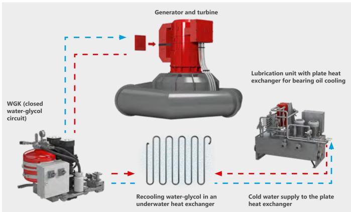
heat the machine cabin or cool the hydraulic fluid. The modular system is specially designed for use in hydropower plants and contains precisely those components that are needed for his purpose.
