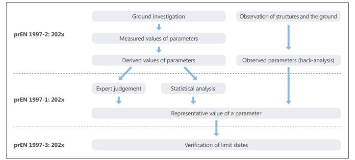
Fig. 5. Sheme for determining the representative value of a soil parameter in the geotechnical design process [9].
