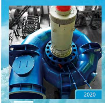
SHP San Secondo, Italy 1x92 kW (d=720mm, H=5.4m)
