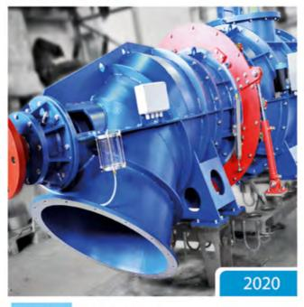
SHP Naviglio, Italy 1x84 kW (d=560mm, H=7.6m)
