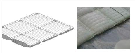
are most often found in use on river banks with susceptible and uncertain substrate. The length of the spacers ranges from 8 to 56 cm, hence the average thickness of the mat can be from 10 to 45 cm. On canals, these mats are used on the excavated sections, i.e. when there may be groundwater inflow into the canal.
